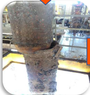
New casing v's very poor condition 20" conductor installed in late 1980's
