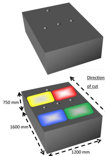
Fig 3: PowerPads within an expanded schematic of the concrete block
