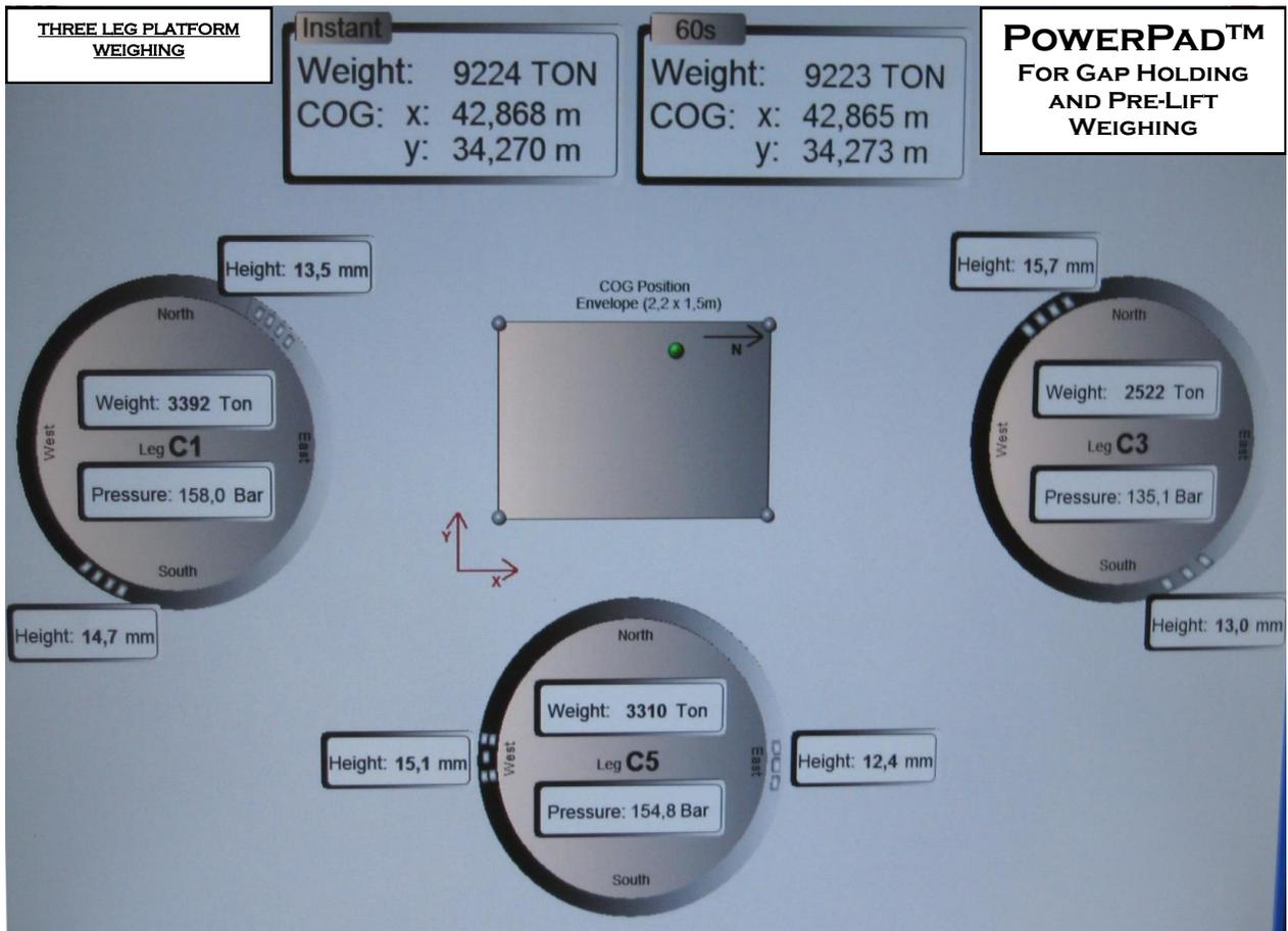
Fig 7. Platform mass and centre of gravity, at the top of the screen display, before lift of a 3 legged platform. The calculated mass, and PowerPad pressure, is within the circles. The heights, within rectangles outside the circles, show the stroke of the inflated PowerPads.
