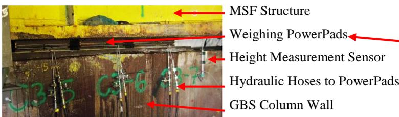
Fig 5: PowerPads and Sensors
