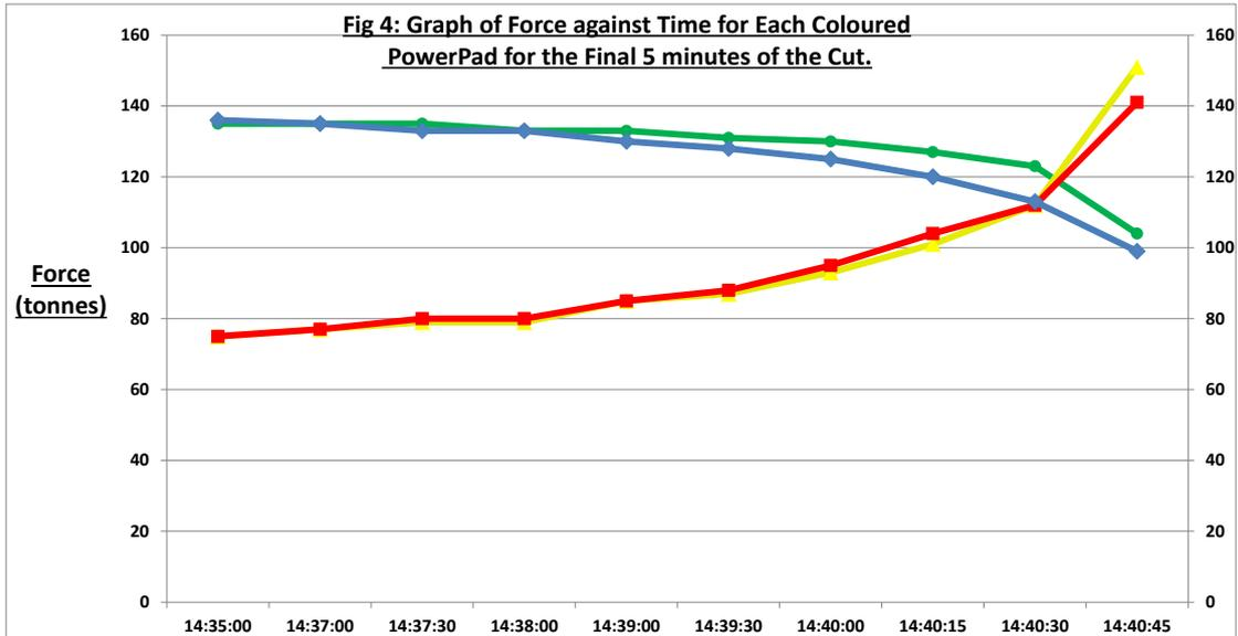
After one hour of cutting, the first two hydraulic pads were inserted and inflated to 40 bar to initiate support of the block and hold open the increasing wire cut gap. At this “activation pressure” the stroke of the pad increased to fill the 11mm gap from the diamond wire cut. The hydraulic fluid volume injected (and locked into the pad) at the start of this “active mode” was approximately 1.4 litres per pad.
